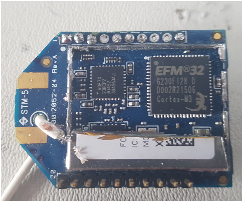
Figure 15 - Exposed Digi S3B Module
